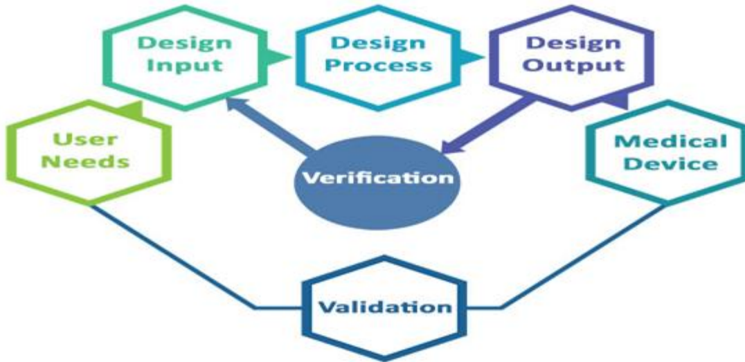
Figure 3: Flow Chart For Medical Devices Process and Production Verification and Validation
