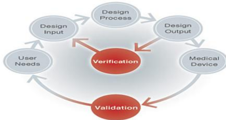
Figure 1: Flow Chart for Validation and Verification
